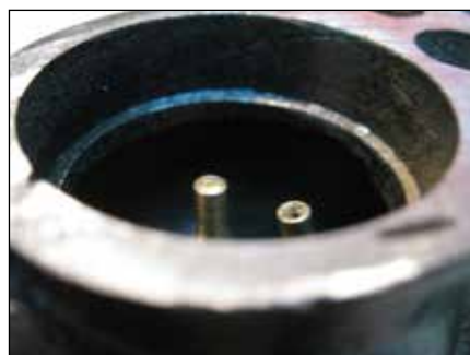
Figure 10. Jet with extra gasket.
