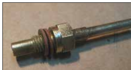
Figure 10. Jet with extra gasket.
