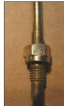
Figure 11. Original jet with stamped number
