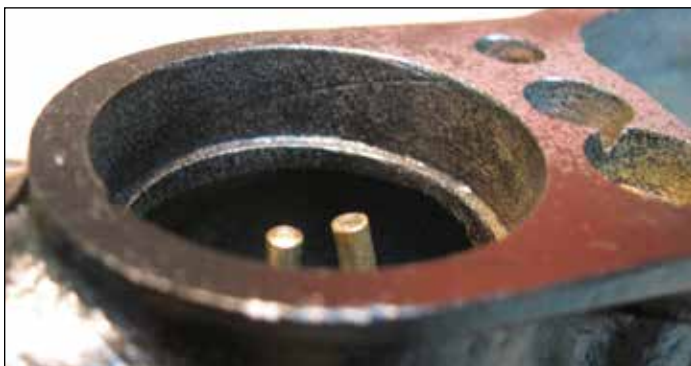
Figure 9. The cap jet stands taller than the main jet.
