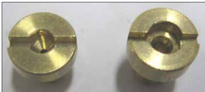
Figure 6. Compensator jet at left adjustment needle set at right.
